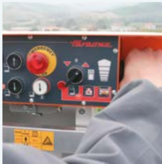
The best you could wish for. Gentle and gradual traction guaranteed by two self-braking drive wheels (with an inactive accelerator) with electric motors managed by a Mosfet PCB. Forget sudden movements, get used to gentleness.
